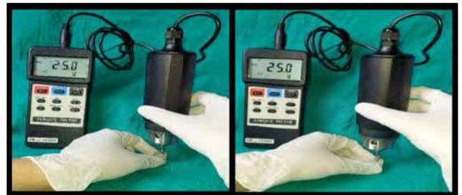
Figure 3: Applying a 25Ncm torque on angulated and straight prosthetic abutment.
